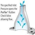
The specified Back Pressure forces the **ProFlex**<sup>w</sup> Rubber Check Valve to close preventing backflow.
